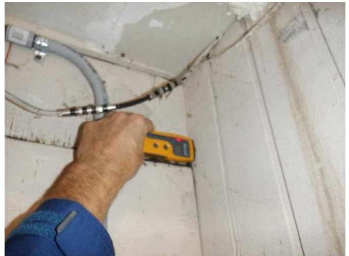
#46 High moisture reading in upper SW corner of garage wall.
