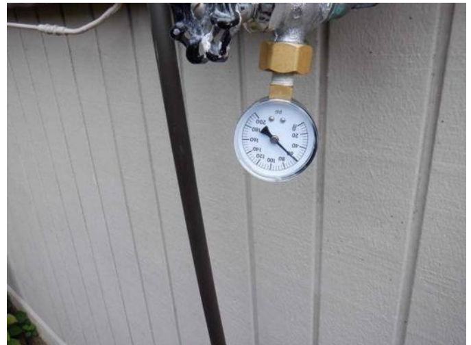
#10 Water pressure tested at 60 psi.
