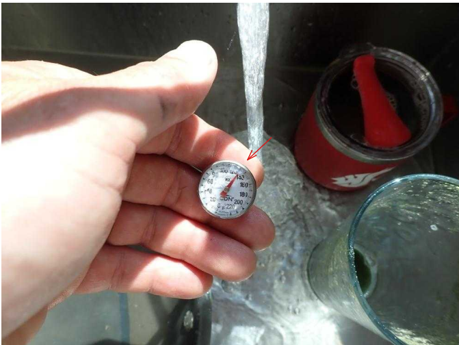
#51 Water temperature is 130 deg F, should be lowered to 120 deg F to reduce the risk of scalding.
