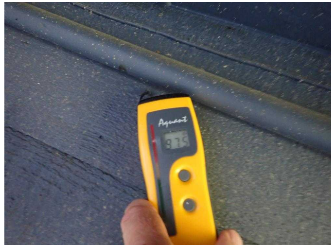
#10 High moisture reading in house siding underneath chimney and in soffit of chimney.
