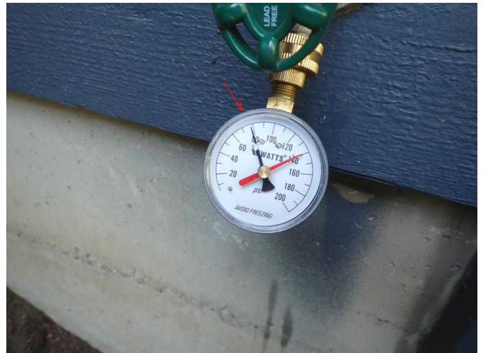
#4 Water pressure 80 psi, acceptable.
